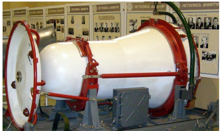
SLBM non-MIRV, weight 650 kg, 1 Mt. Put in service in 1974.
